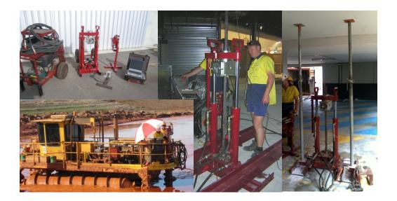
Our 200kN portable pushing frame is great for hard to access areas including underground carparks and indoor testing.
